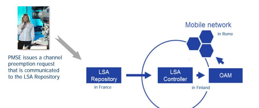
The evacuation time is the time needed to reconfigure the LTE network so to make the channel available for the PMSE user.
