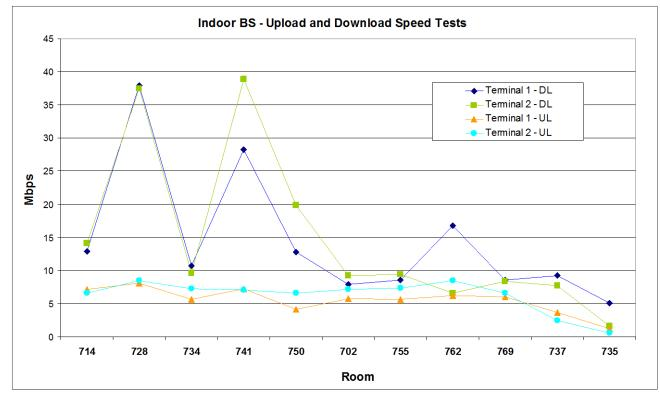
A strong fluctuation of the measured download bit rate has been registered in the different locations
