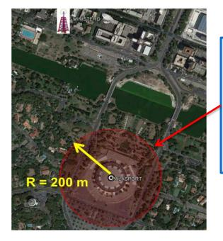
The mean field strength, within the protection zone, shall not exceed a defined value in dBµV/m/MHz at a defined receiver antenna height above ground level
